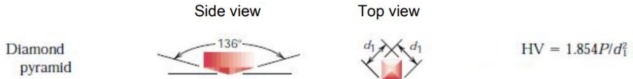
Fig. 3-16: Vickers hardness testing technique
